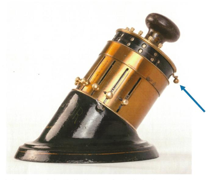
Don't use the <u>reset mechanism</u> at the side of the upper part, because it doesn't work anymore and machine blocks.
